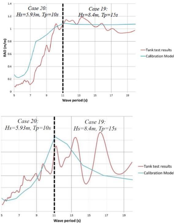
Figure 2. Comparison of motion RAOs from simulations (in blue) to tests (in red) – Heave (top) Pitch (bottom)
