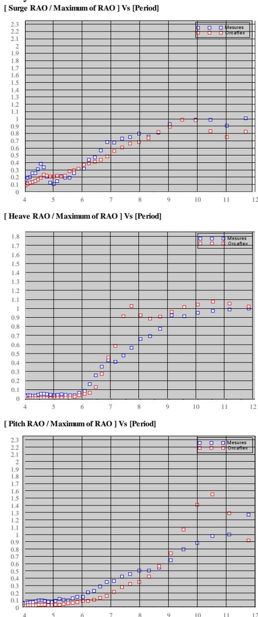
Figure 6. Comparison of measured and calculated Surge (Top), heave (middle) and pitch (bottom) RAO Amplitudes are scaled to the maximum of the measured value.
