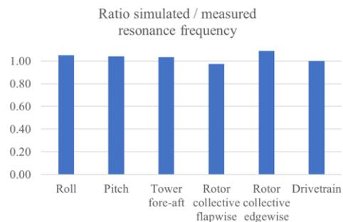
Figure 5. Comparison of natural frequencies as measured during power tests in port to simulations
