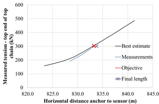
Figure 8. Load/extension curve during hook-up
