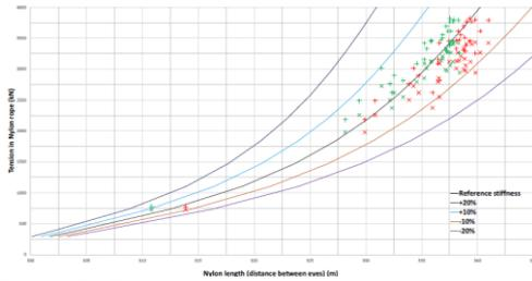
Figure 7. Pull-in test load/extension curve during installation
