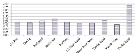
Figure 5. Ratio of loads [floating/fixe] turbine.
