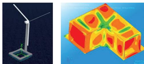
Figure 8. Hull verification models global model (left) and local model (right)
