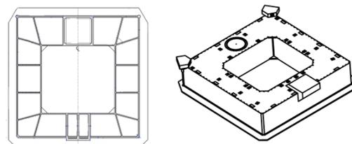
Figure 7. Hull Structural arrangement
