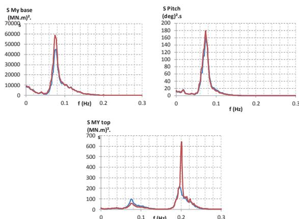
Figure 3. Comparison of response spectra for tower base moment (top left), pitch (top right), tower top bending moment (bottom). The blue curve is the measurement in combined wave / wind conditions and the red curve is the sum of spectra measured in the corresponding wave-only and wind-only model tests.
