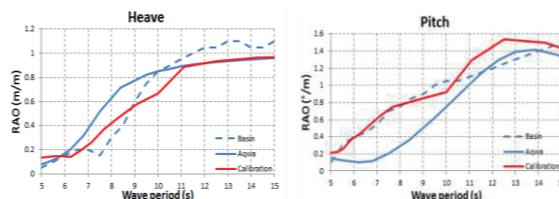
Figure 4. Comparison of measured (dashed) and calibrated (red) motion transfer functions. The Blue solid line stands for diffraction-radiation models.
