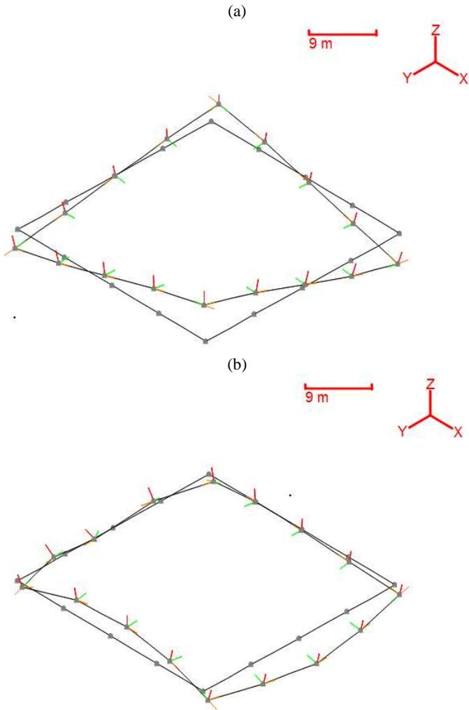
Fig. 6. First vertical hull bending moment (a) and first horizontal bending moment (b) floater deformation mode computed by OrcaFlex at respectively 0.213s and 0.201s. Only the beams linking the compartments and their local axis are drawn.
