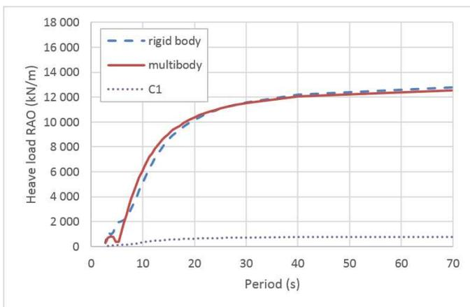
Fig. 3. Heave Response Amplitude Operator for rigid body model, C1 compartment (below the tower) and multibody model (sum of all compartments contributions).
