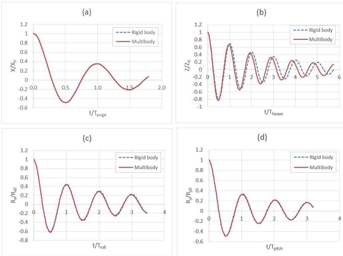
Fig. 4. Dimensionless decay tests in (a) Surge; (b) Heave; (c) Roll and (d) Pitch for multibody and rigid body models. Time is divided by rigid body natural period and displacement by initial amplitude of movement.
