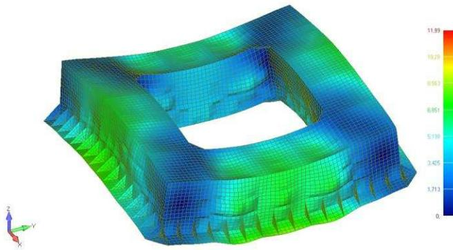
Fig. 10. Floater finite element model as used for the structural analysis. Local deformation is presented for the static case.
