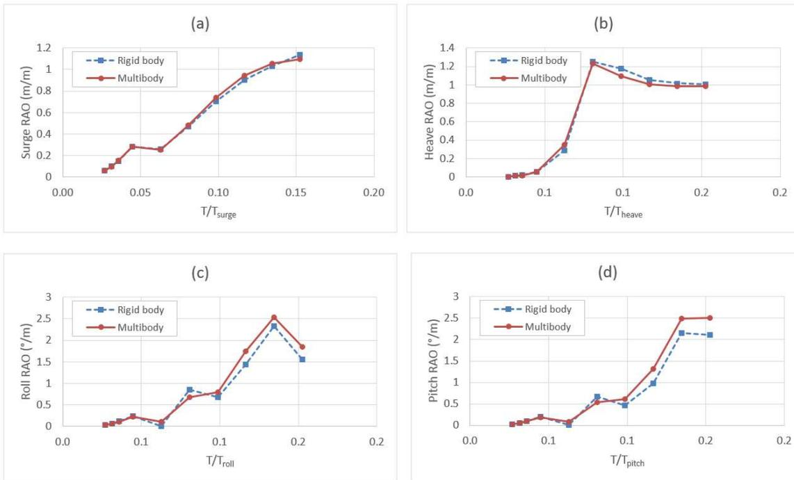
Fig. 5. Response Amplitude Operator for rigid body and multibody models for four degrees of freedom: (a) surge, (b) heave, (c) roll and (d) pitch. Incident wave period is divided by rigid body natural period. The Airy waves heading is  $180^{\circ}$  for surge, heave and pitch and  $90^{\circ}$  for roll degree of freedom. RAO are calculated at floater centre of gravity.
