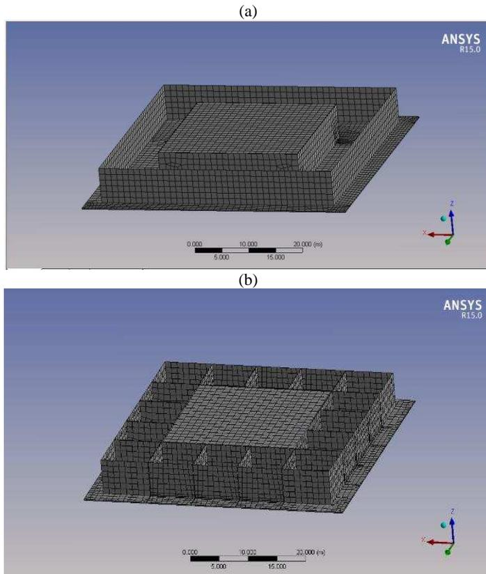
Fig. 2. View of the meshed floater as rigid body (a) and multibody (b)
