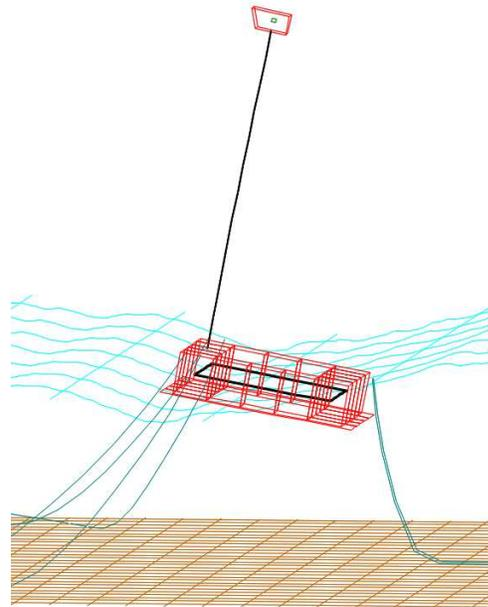
Fig. 8. View of the OrcaFlex model of the floater in one of the critical case. The turbine is idling, wind is coming from the aft of the floater and waves are coming from the front. The platform presents a 10.7° pitch angle.
