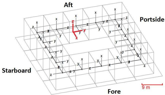
Fig. 7. Global axis of the floater (in bold red) and local axis of the beams (in thin black).
